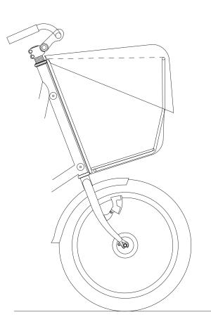
3. Put the wood base panel on the bottom side of the bag (over the metal arch)
